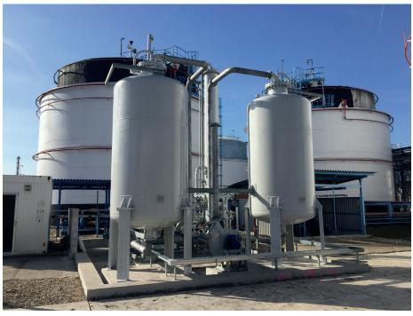
Figure 6 - Vapour recovery unit based on activated carbon and absorption. Cool Sorption, 2019
