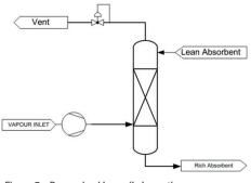
Figure 7 – Pressurised lean oil absorption
