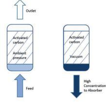
Figure 4 – Principle of activated carbon system
