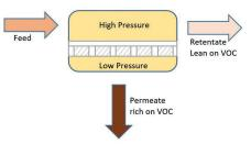
Figure 3 – Principle of membrane system
