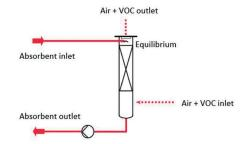
Figure 2 – Diagram of a scrubber
