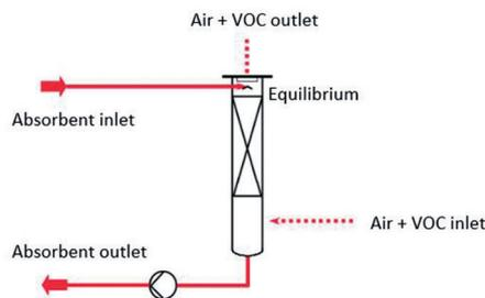
Figure 2 – Diagram of a scrubber
