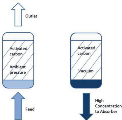
Figure 4 – Principle of activated carbon system
