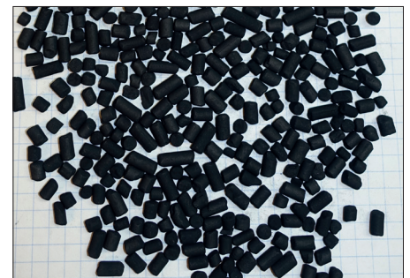
Activated carbon pellets with too many short pellets and inconsistent pellet diameters
